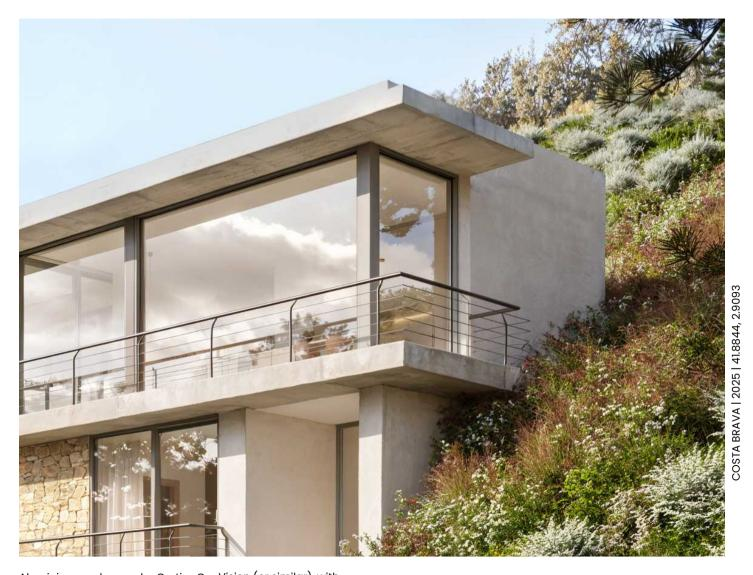
Aluminium enclosures by Cortizo Cor Vision (or similar), with concealed track system in the dining area, featuring double glazing on sliding doors and windows.
